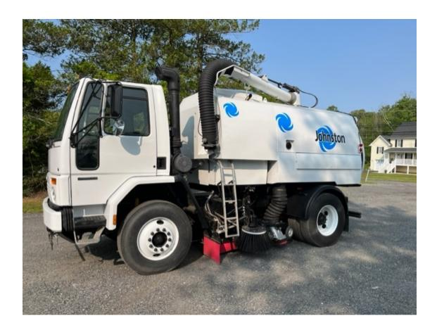
This Johnston sweeper is mounted on a 2001 Sterling SC7000 Cab over chassis with only 54,000 miles. The truck is powered by a 6cylinder Cummins Diesel engine, Allison AT545 automatic transmission, and air brakes. Dual Steering, dual gauges and air conditioning are included.
